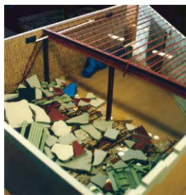
Winery deck collapse – wrongful death and personal injuries 1:12 scale
